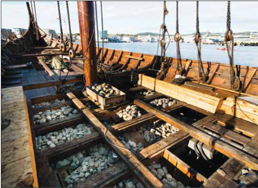
Draken is ballasted with stones, which were loaded and shifted by hand.
