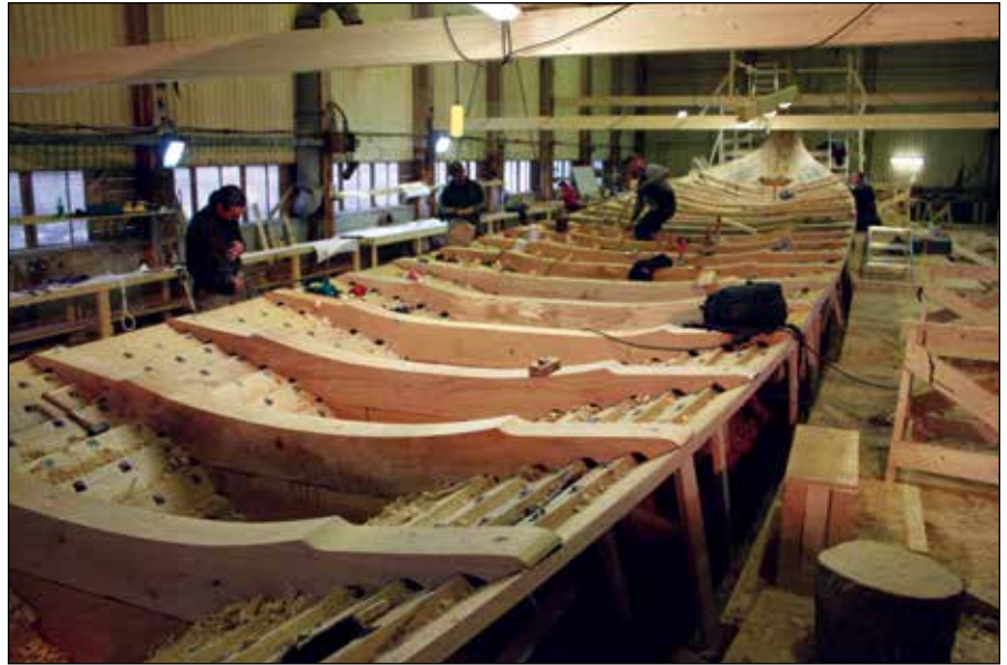
Draken Harald Hårfagre being built in Norway. This photo shows some of the laborious notches and curves that the shipbuilders had to contend with in her construction.
