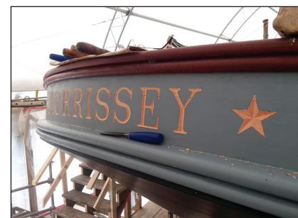
With the first phase of her restoration nearing completion, it was time to carve her name back into her rebuilt stern.
